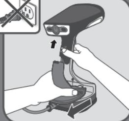
**EN** Unlock and remove the water tank.
