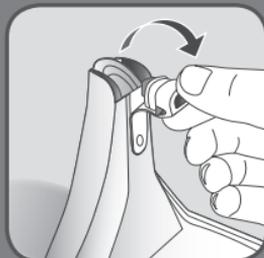
**EN** Remove the water inlet stopper.
