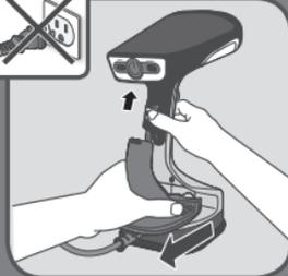
**EN** Unlock and remove the water tank.
