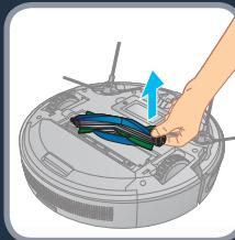
**EN** Clean the brush of the robot once a week. To do that turn the robot upside down. To remove the brush, open the brush guard by pushing the 2 snap latches and pull it up. Then pull out the brush from the robot.
