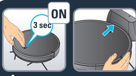
**EN** To charge the robot turn it on by pushing the on / off button for 3 seconds. Place the robot on the docking station: the charging plates on the robot must touch those on the docking station. Replace the robot on its charging base after use.
