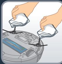
**EN** To clean the brush, use the cleaning accessory or scissors to cut away any hairs. Clean the robot's side brushes with a clean, dry cloth at least once a month.
