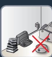
**EN** To place the docking station, make sure there is an empty area of 1.5m on each side and 2m in front of the docking station. Do not install the docking station near stairs. The cable must be tight. Always place the docking station on hard floor. Do not place the docking station on carpet.
