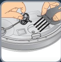
**EN** To clean the wheels, clean the front, left and right wheels regularly with a cleaning brush. The wheel shaft may be entanglement by hair, cloth strips, etc. so please clean it in time.
