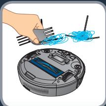
**EN** To clean the side brush, remove it and use a cleaning brush to clean the side brush and the entanglements in the slot of the side brush. Replace lateral brushes every 6 months.
