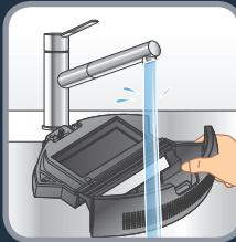
**EN** Clean the filter cover and the filter by tapping the back, holding it above a waste bin. Wash the foam filter, the filter cover and the dust catcher in clean water. Do not wet the fine dust filter (white filter). The filters must be cleaned at least once a week.
