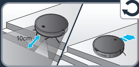
**EN** The robot has drop sensors to detect stairs and gaps. The robot will change direction when detecting them. In order to correctly detect the floor level difference, make sure there are no objects (bags, shoes...) on the floor next to gaps, stairs or on the stairs' steps. The step must be more than 10 cm away to be detected.
