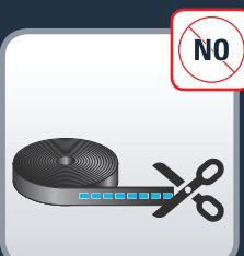
**EN** Should you like to restrict access of the robot to some areas, use the magnetic stripe. Put the magnetic stripe on the floor to mark a no-go zone for the robot.
