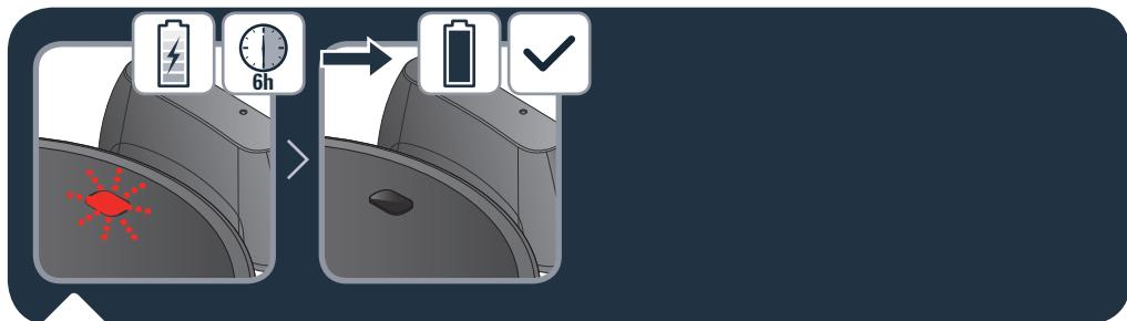
**EN** When the on/off button blinks the robot is charging. Once the on / off button stops blinking it is fully charged (6h for the battery to be fully charged).
