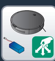
**EN** Attention: Before removing the battery turn off the robot. Turn the robot upside down to get access to the battery slot. Remove the battery by pressing snap latches of the battery slot and pull the battery up. Disconnect the battery from the robot. Recycle the battery and robot.
