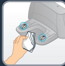
**EN** Once a week, clean the following parts with a clean, dry cloth: the robot's charge plates, fall sensors, distance sensor, the docking station's charge plates and the robot's front wheel.
